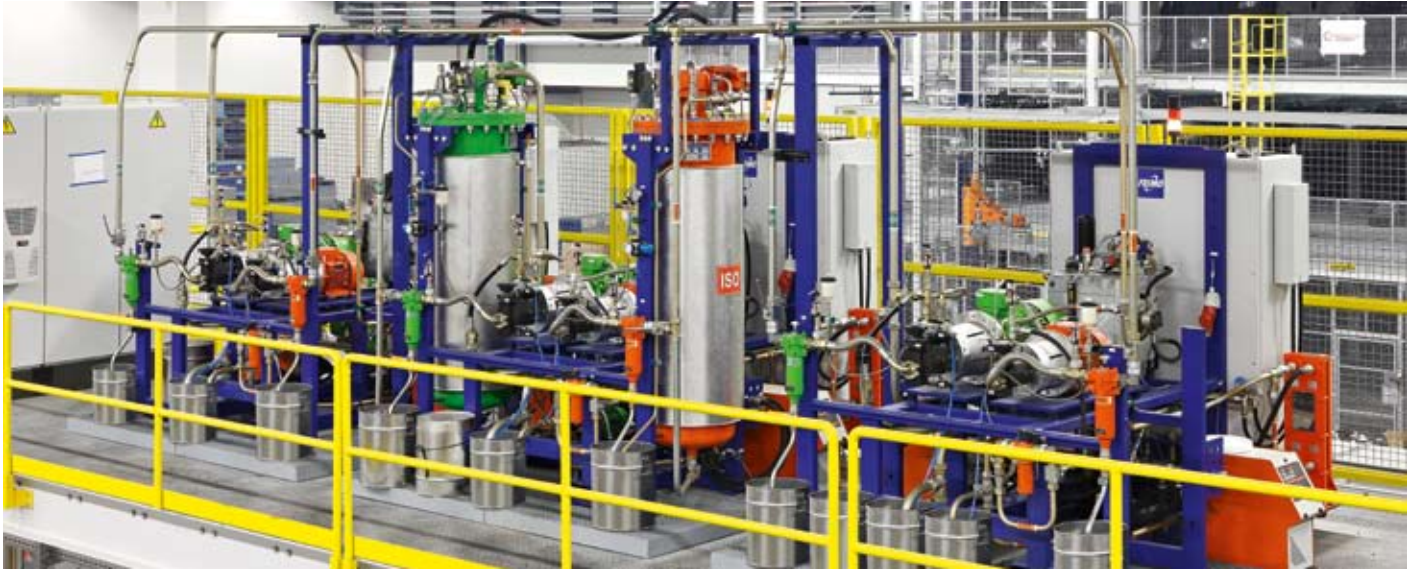
FRIMO PURe Line multi-component dosing with centralized raw material supply
